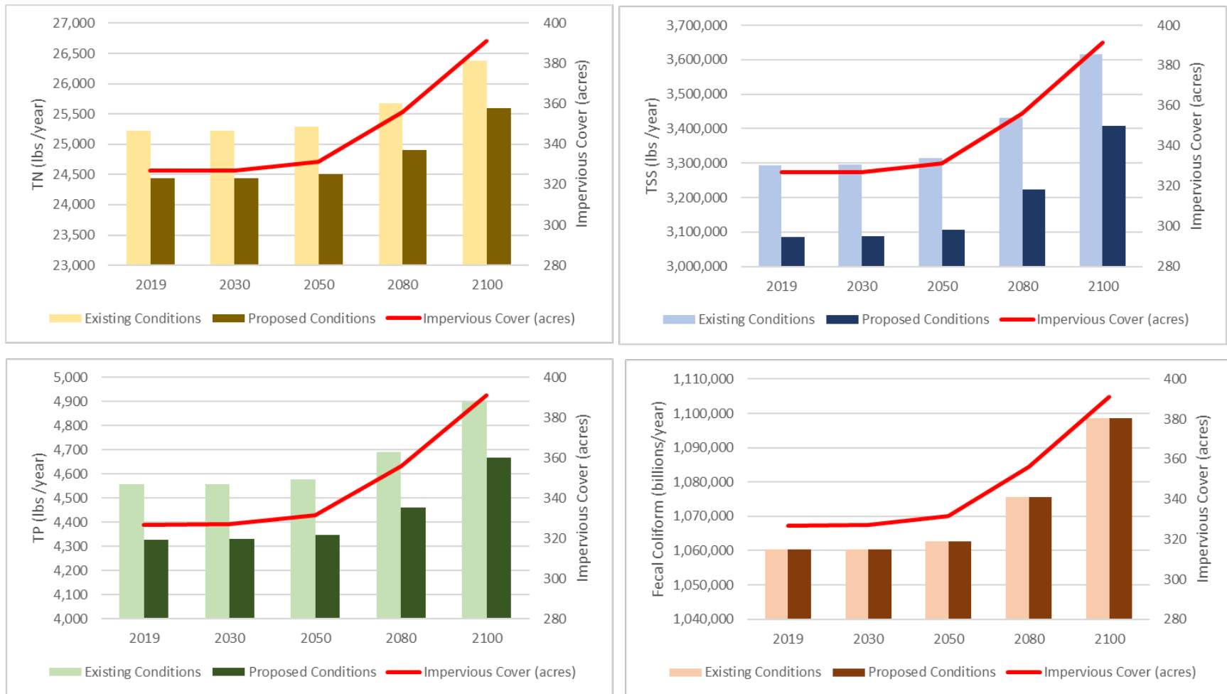
Figure 81. Relationship over time between watershed scale pollutant loading for the existing conditions (lighter colors) and proposed conditions (darker colors), which includes the implementation of the Top 10 BMPs. Loading is shown for TN (yellow), TSS (blue), TP (green), and Fecal Coliform (orange). The predicted impervious cover increase (red line) over time is also shown.
