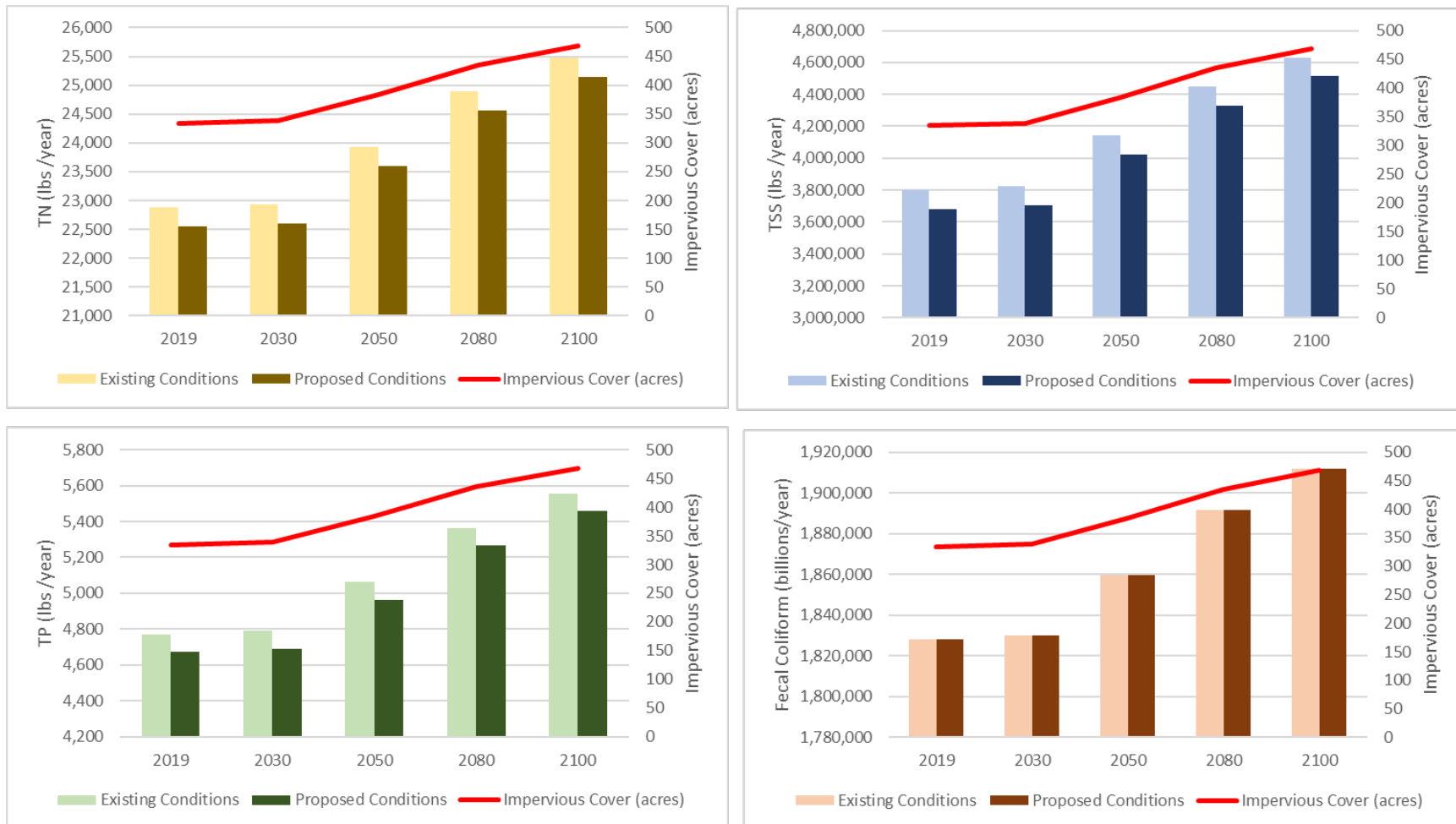
Figure 88. Relationship over time between watershed scale pollutant loading for the existing conditions (lighter colors) and proposed conditions (darker colors), which includes the implementation of the Top 10 BMPs. Loading is shown for TN (yellow), TSS (blue), TP (green), and Fecal Coliform (orange). The predicted impervious cover increase (red line) over time is also shown.
