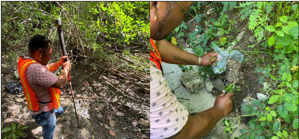
Figure 55. A sediment core being collected from the LPB01 gut channel (left) and a subsample of sediment being collected from the LPB03 gut channel (right).
