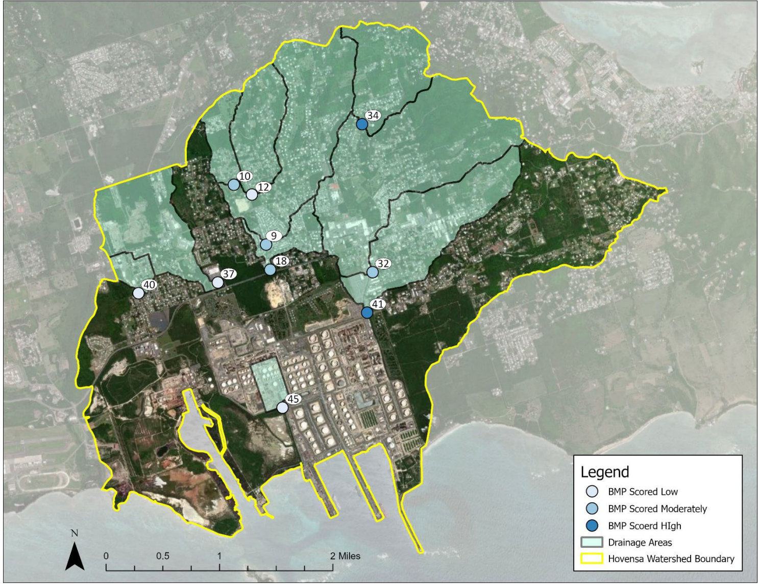
Figure 80. Depiction of the relative ranking of each BMP and the associated BMP drainage area. Note that the drainage areas of several of the identified BMPs overlap.
