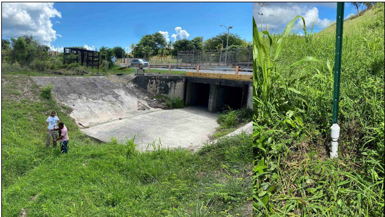
Figure 58. Field crew member setting up an Onset HOBO U20 Water Level Logger at gauge station STH 01 (left). A closeup of the monitoring configuration at Hov02 (right).
