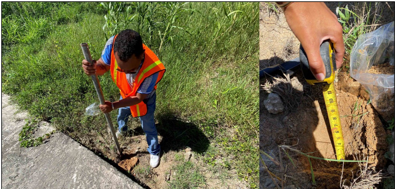
Figure 59. A sediment core being collected from the Hov02 gut channel (left). The depth of the extracted sediment core verified with a tape measure (right).
