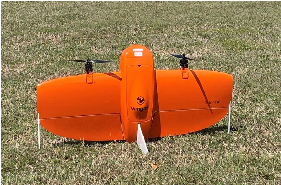
Figure 53. WingtraOne Gen II UAS utilized to collect data in the study watersheds.
