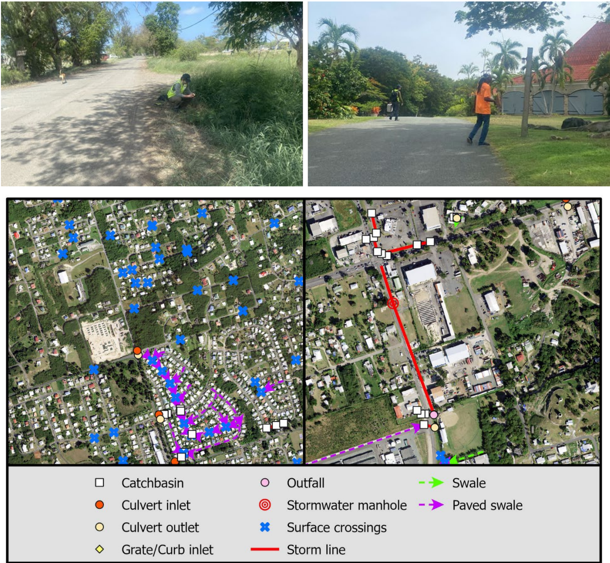
Figure 50. Inspection of existing stormwater infrastructure during field assessments (above) and an example of the maps produced (below).
