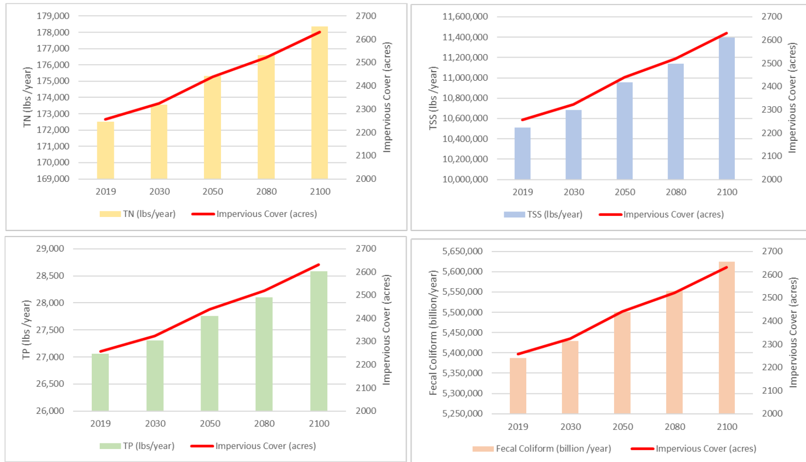
Figure 87. Relationship between watershed-scale pollutant loading for TN (yellow), TSS (blue), TP (green), and Fecal Coliform (orange) and the predicted impervious cover increase (red) over time
